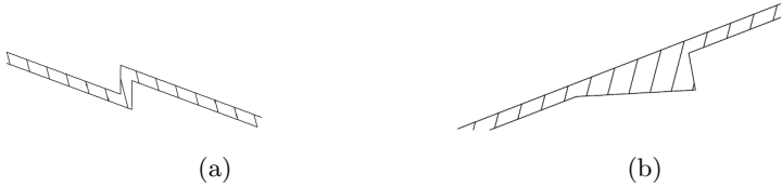
Figure 5: Difference in cross section of (a) deflector and (b) spray rail
